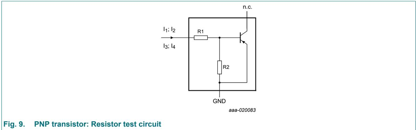
Fig. 9. PNP transistor: Resistor test circuit
