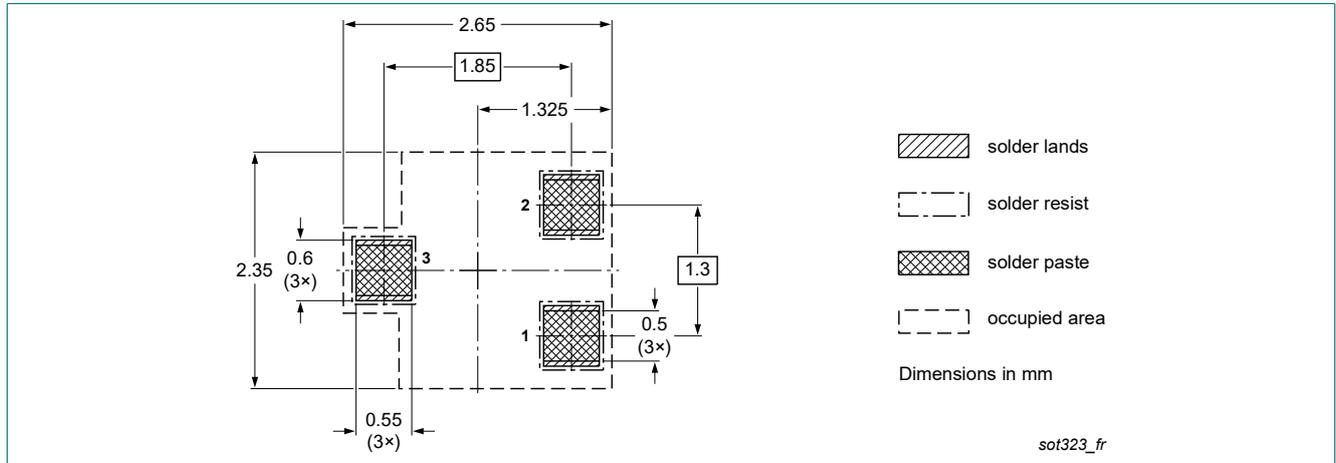
Fig. 11. Reflow soldering footprint for SC-70 (SOT323)
