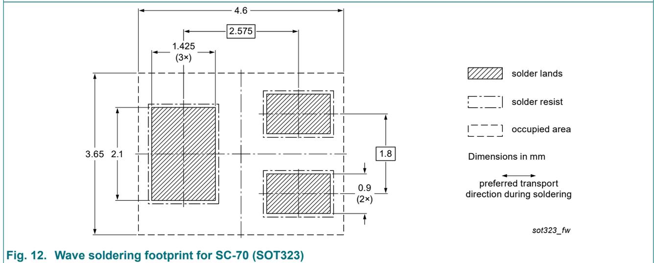
Fig. 12. Wave soldering footprint for SC-70 (SOT323)
