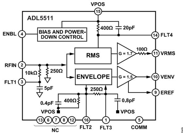
Figure 48. Block Diagram
