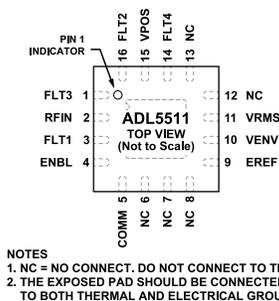
Figure 3. Pin Configuration
