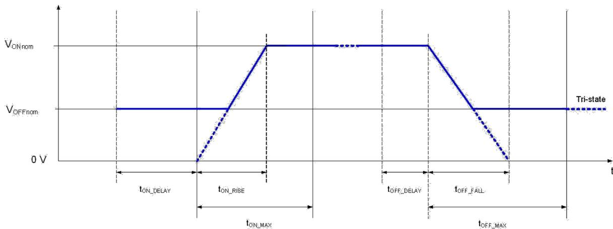
**Figure 8: Power Sequencing With Non-Zero Off Voltage**
