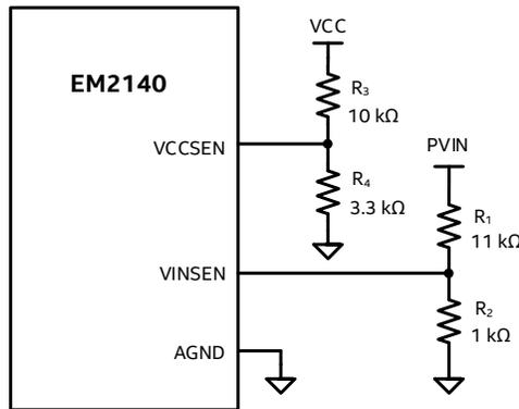
**Figure 4: VINSEN And VCCSEN Input Resistor Dividers**
