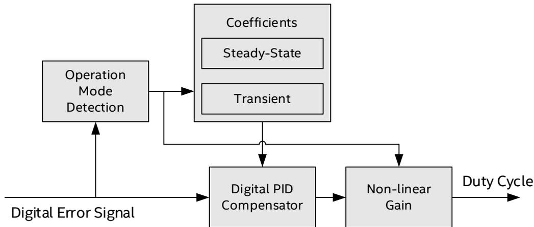
**Figure 3: Simplified Block Diagram Of The Digital Compensation**
