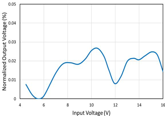
EM2140 Load Regulation,  $V_{OUT} = 0.9V$
