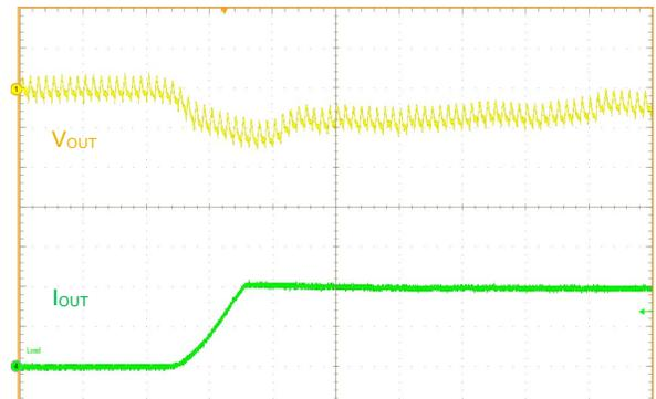
$V_{IN} = 12V, V_{OUT} = 0.9V, 10 \mu s/div$
