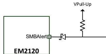
**Figure 7: SMBAAlert Pin Low Voltage Pull-up Option**
