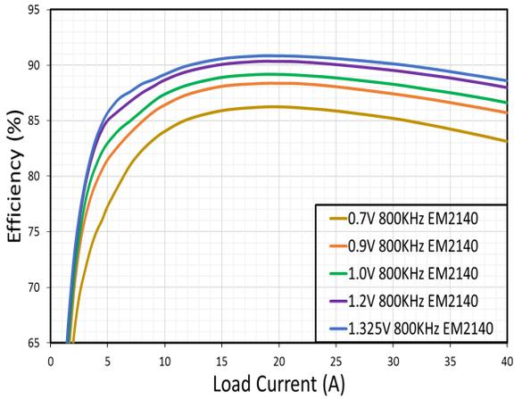
Efficiency,  $V_{IN} = 5V$
