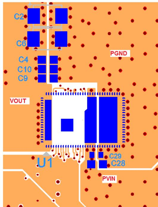
**Figure 16: Top Layer Layout With Critical Components Only**
