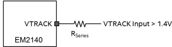
Figure 12: VTRACK Sense Circuitry (Input > 1.4V)
