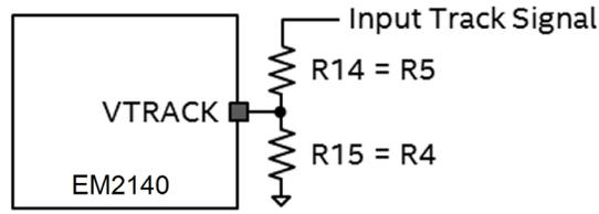
Figure 11: VTRACK Sense Circuitry with Resistor Divider
