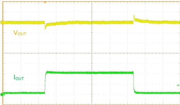
$V_{IN} = 12V, V_{OUT} = 0.9V, 100 \mu s/div$
