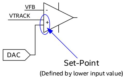
**Figure 10: VTRACK Circuitry**
