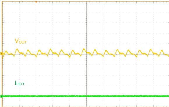
$V_{IN} = 12V, V_{OUT} = 0.9V$
