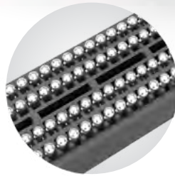
Solder ball technology for simplified processing
