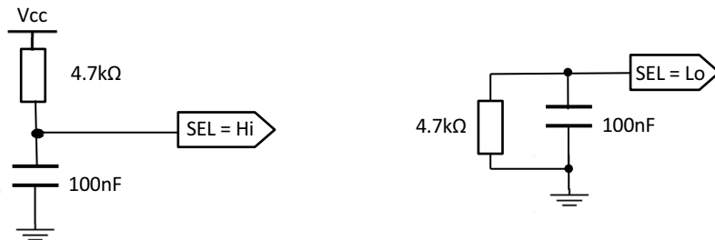
Figure 5: Examples of High and Low Selection Circuits
