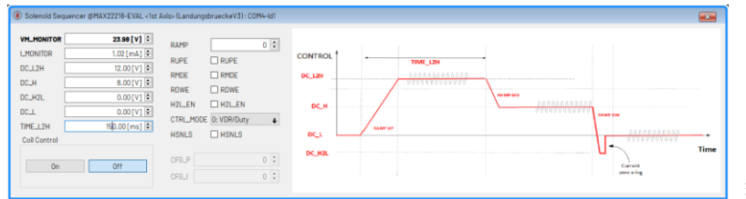
Figure 10. Channel 0 > Solenoid Sequencer: Example Setup for 12V Solenoid (VDR Full-Bridge Mode)
