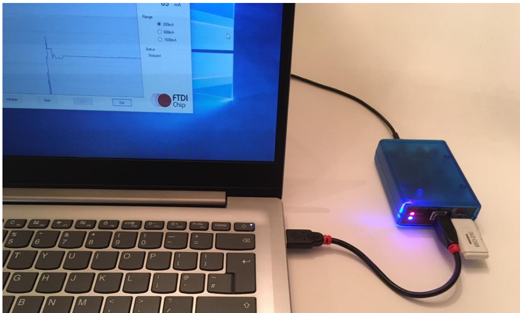
Figure 15 - Connecting the meter to the link under test
