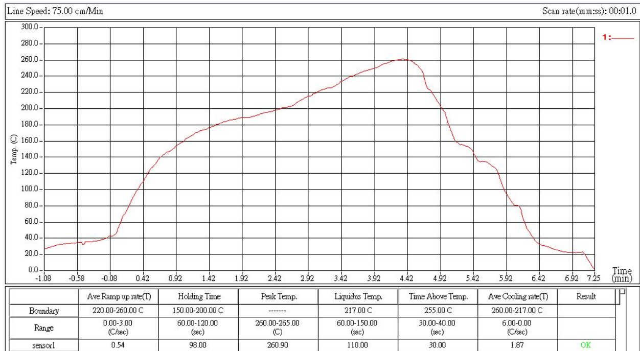
Figure 8.5 Solder Reflow Profile
