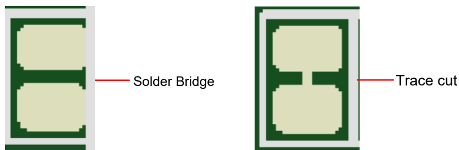
Figure 6-1 Solder Bridge and Trace Cut
