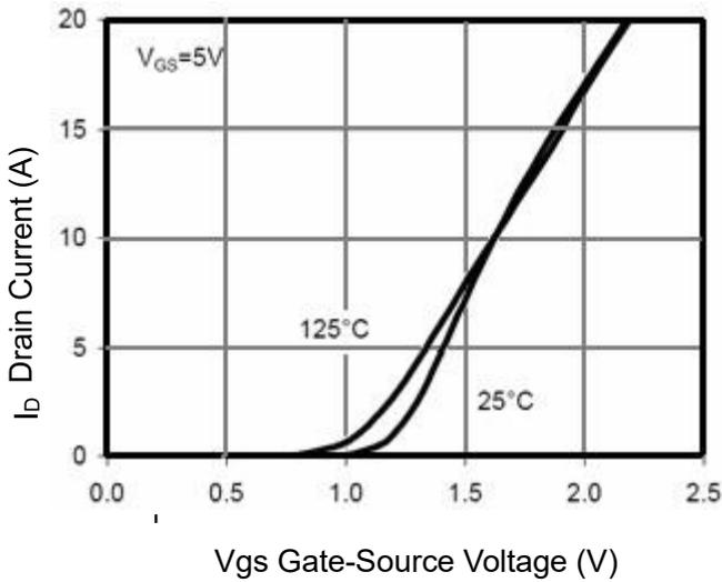
**Figure 7 Transfer Characteristics**
