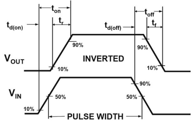
**Figure 2: Switching Waveforms**
