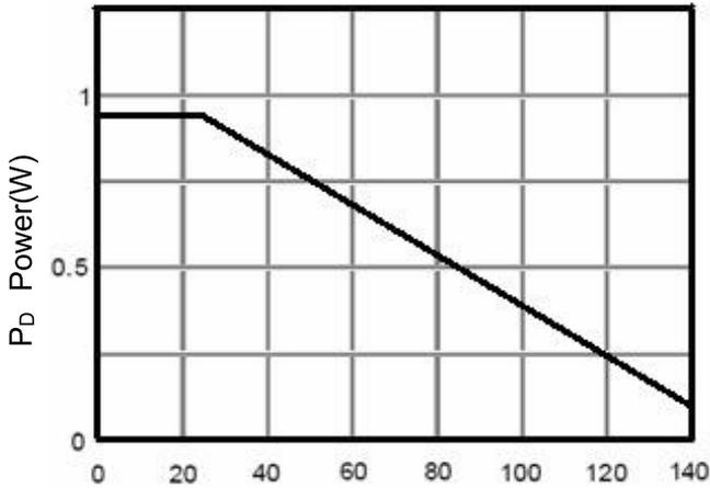
**Figure 3 Power Dissipation**
