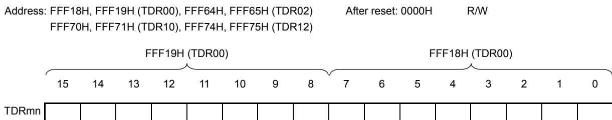
Figure 7 - 8 Format of Timer data register mn (TDRmn) (n = 1, 3)
