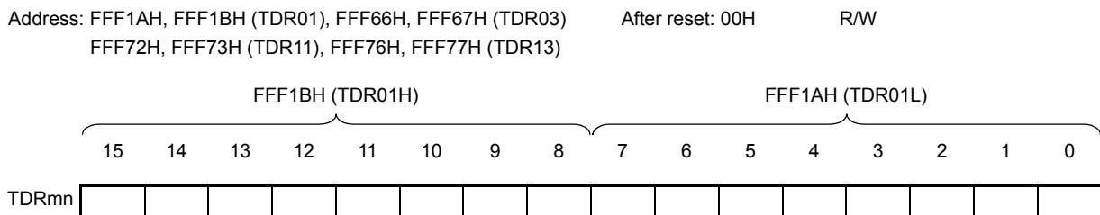
Figure 7 - 8 Format of Timer data register mn (TDRmn) (n = 1, 3)
