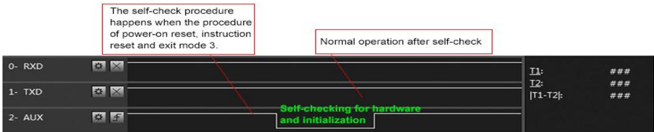
Timing Sequence Diagram of AUX when self-check
