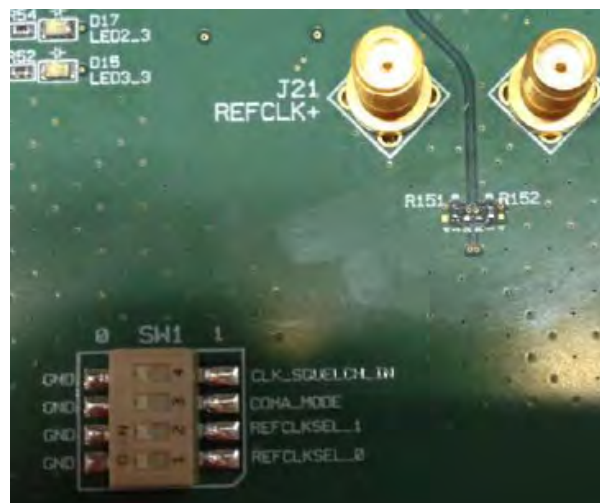
Figure 2 • SW1 Switch Control
