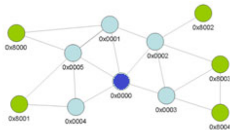
Figure 1-1. Typical Lightweight Mesh Network Application Scenario
