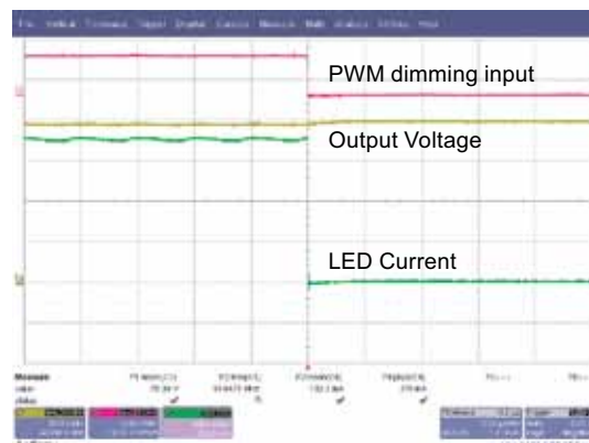
Fig. 8b: Fall time of LED Current at 80V output (5 \mu s/div)
