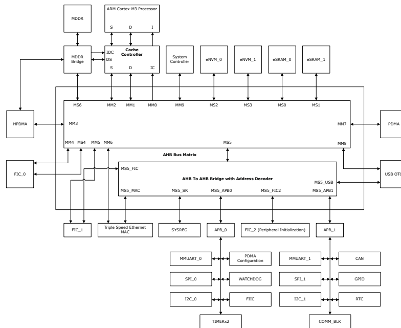
Figure 1-1. SmartFusion 2—System Controller Interfacing with AHB Bus Matrix
