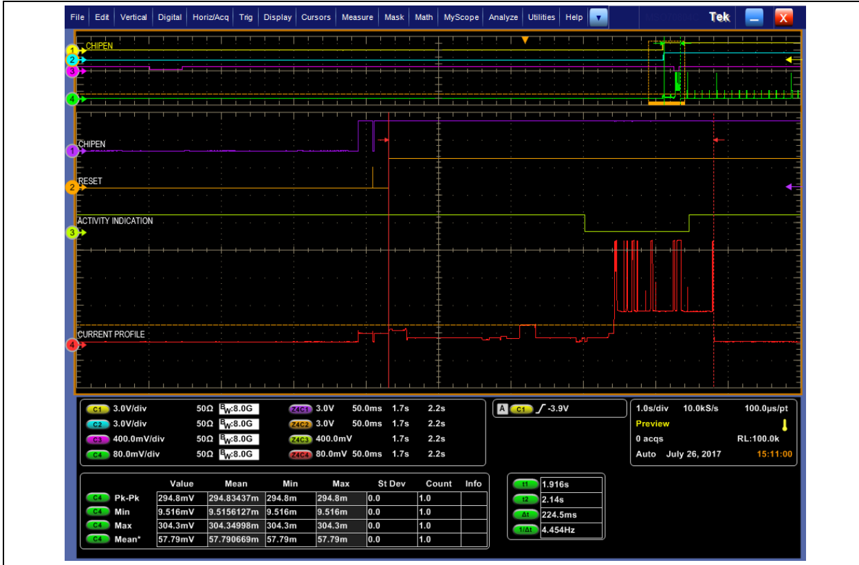
FIGURE 10: WINC TIME AND POWER PROFILE FROM BOOT TO CONNECTION WITH THE AP
