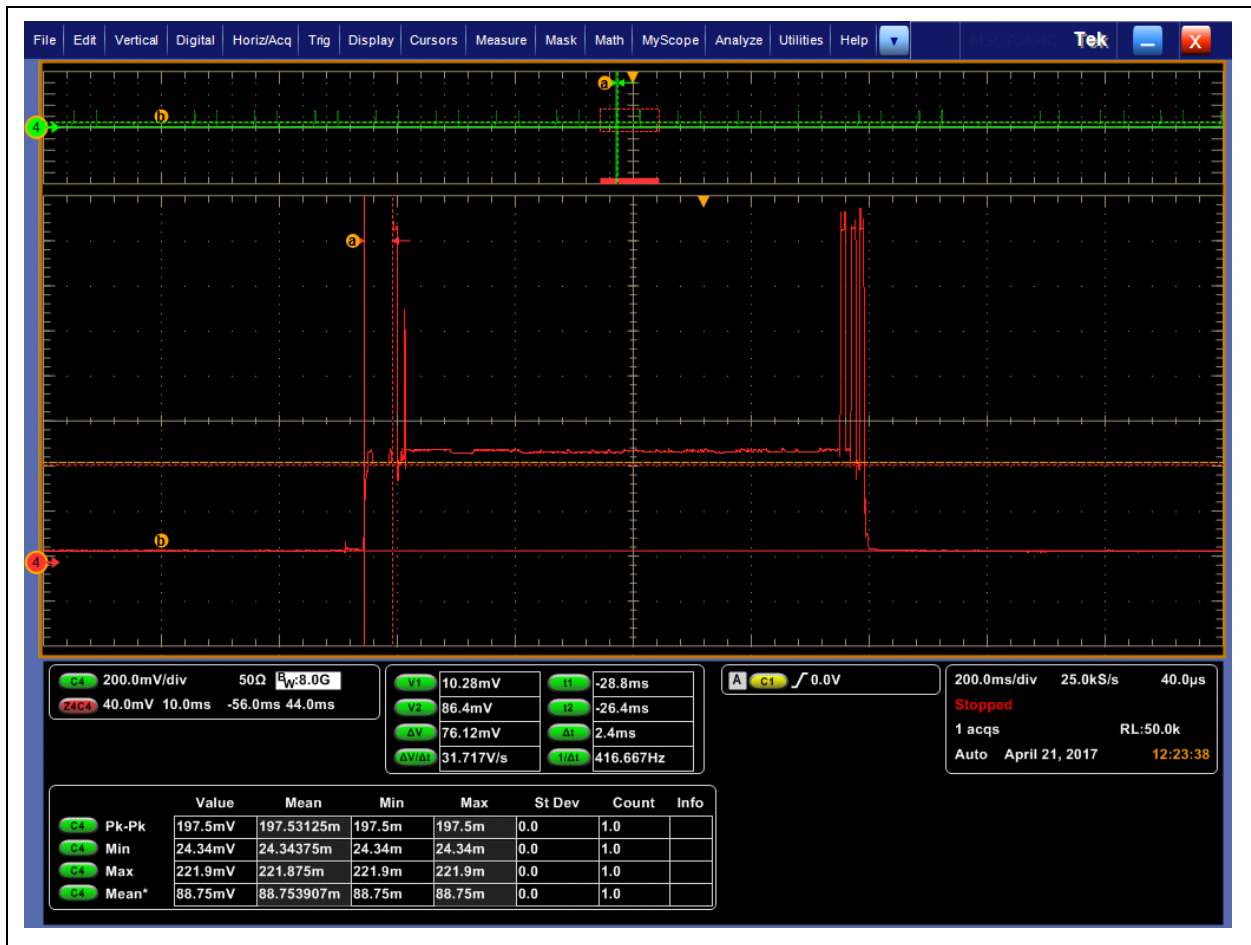
FIGURE 8: WINC1500 RECEIVING 1024 BYTES OF UDP UNICAST PACKET, \Delta t SHOWN HERE IS THE TIME BETWEEN WINC WAKE UP AND SENDING NULL FRAME
