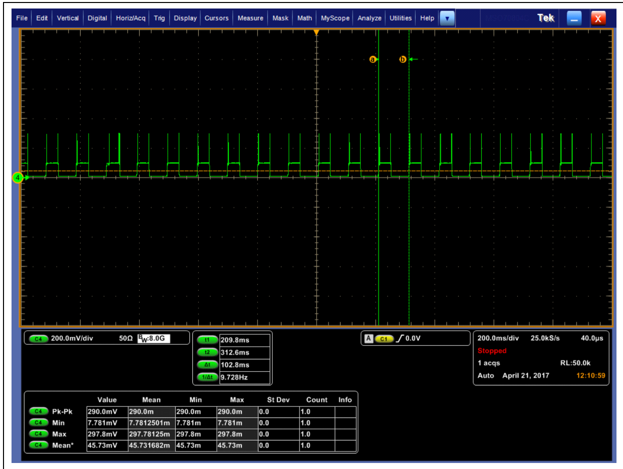
FIGURE 7: WINC1500 WAKING UP EVERY BEACON INTERVAL TO RECEIVE DATA FRAME FROM THE AP
