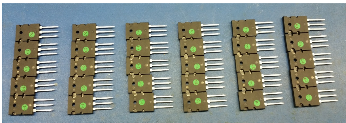
Figure 9 Randomly Selected Devices, Five Each from Six V_{th} Gain BINs
