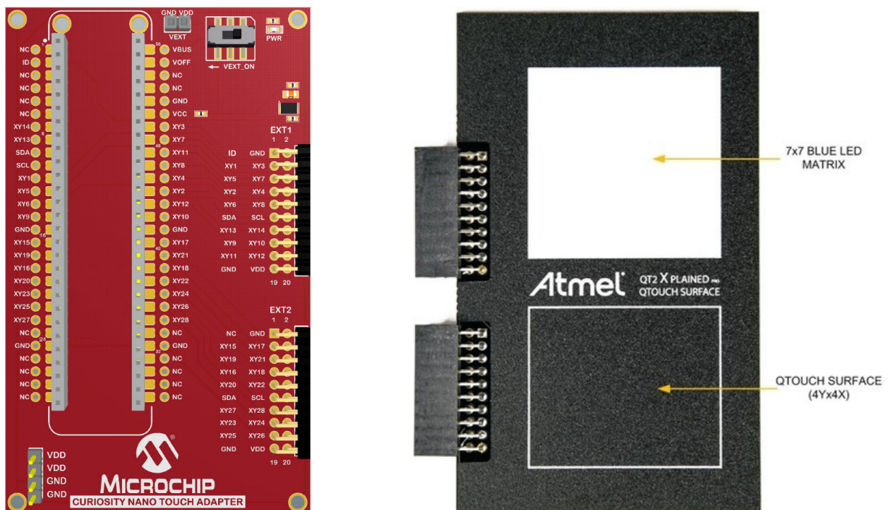
Figure 6-1. AVR128DA48 Curiosity Nano Touch Adapter Board, QT2 Xplained Board, and AVR128DA48 Curiosity Nano
