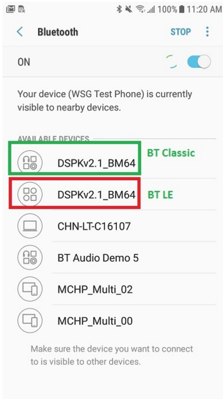
Figure 1-14. Scanning the Devices
