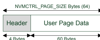
Figure 3-2 Internal Layout of An Emulated EEPROM Page
