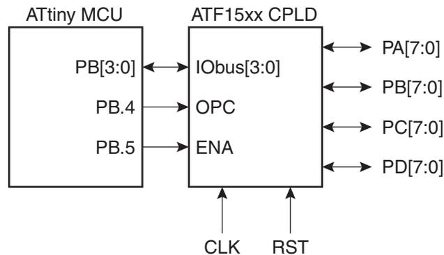
The provided AVR assembly source file (IOexpT13.asm) increments an internal counter and outputs its value to CPLD\_PortA which is configured as output port. Minor modifications are required to use the assembly source with other AVR MCUs. In most cases, the available MCU port may need to be changed as well as interrupt vector table and the stack location (since ATtiny13 does not use SPH register).
