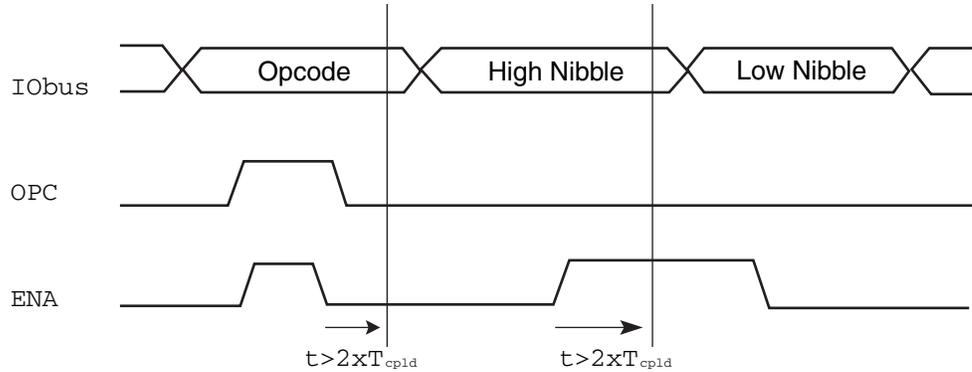
**Figure 4-3.** MCU Extending IObus Output While Reading an Input Port
