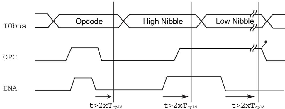
Regarding the I/O Expander implementation, the core of the design consists of a state machine with six states. Two states are required for sending/receiving each nibble, while an additional one is necessary for decoding the opcode. More details about the design are provided by the in-line comments that accompany the VHDL and the assembly source code files.
