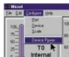
Figure 8. Turning on Power to the Evaluation Board
