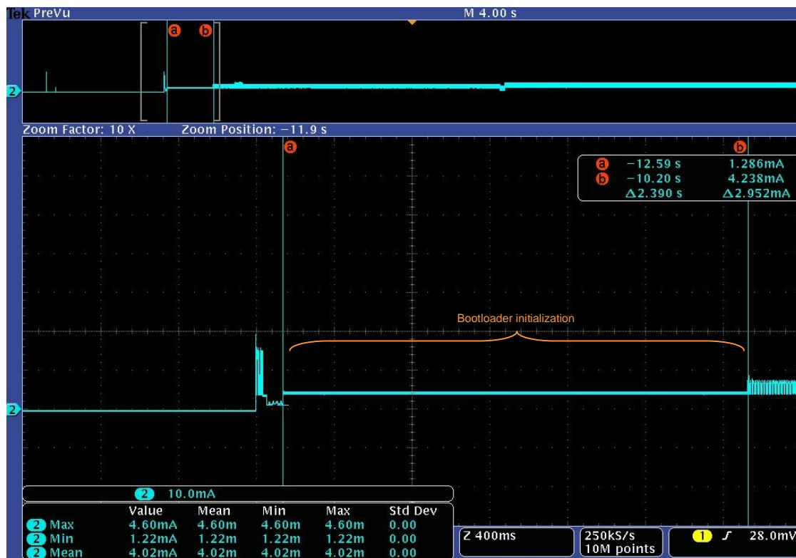
Figure 13-28. Current Consumption Profile of Bootloader Initialization at 16MHz
