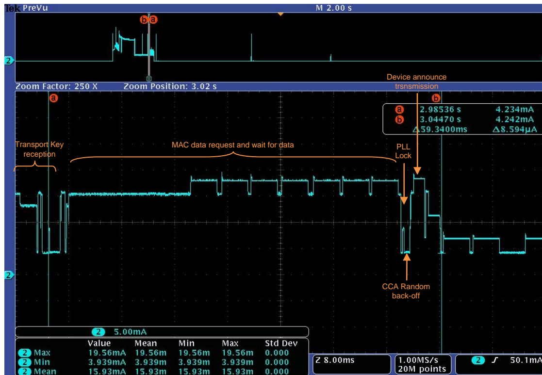
Figure 9-11. Current Consumption Profile of Device Announce Transmission at 16MHz
