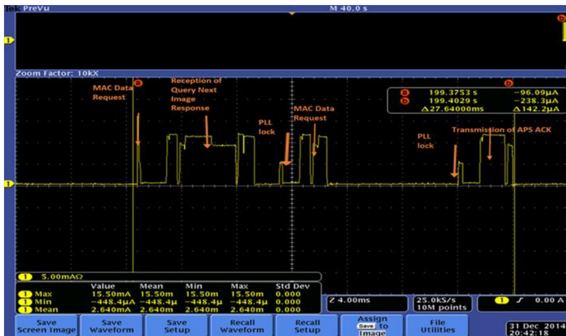
Figure 13-8. Current Consumption profile of Query Next Image Response at 8MHz
