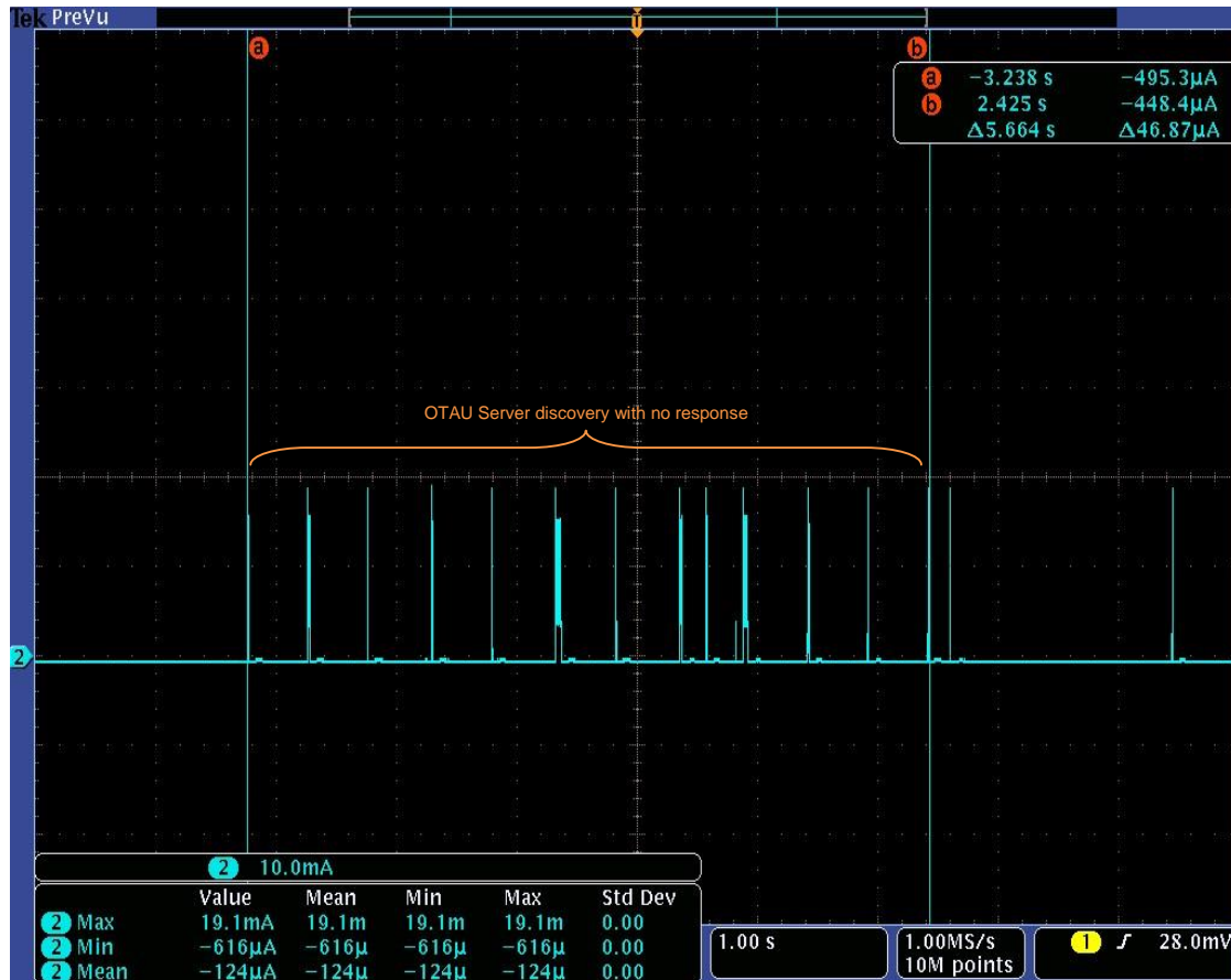
Figure 13-3. Current Consumption Profile of OTA Server Discovery with no Response at 16MHz
