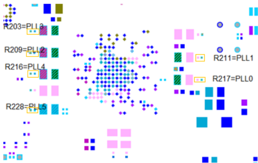
Figure 13 • Bottom Side Location of Series Resistor for FPLL Power Supplies
