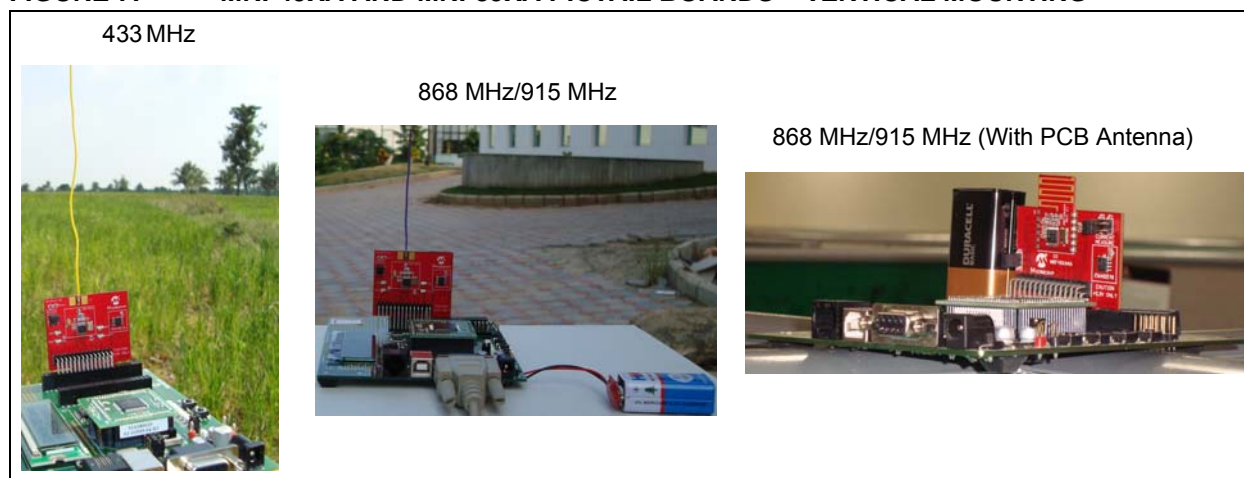
FIGURE 7: MRF49XA AND MRF89XA PICTAIL BOARDS – VERTICAL MOUNTING
