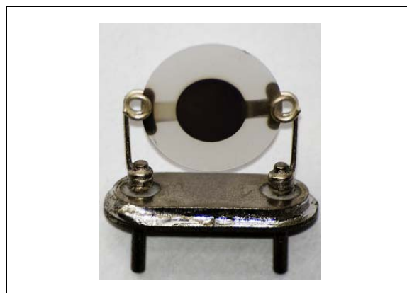
FIGURE 2: Traditional Construction of a Quartz Crystal.
