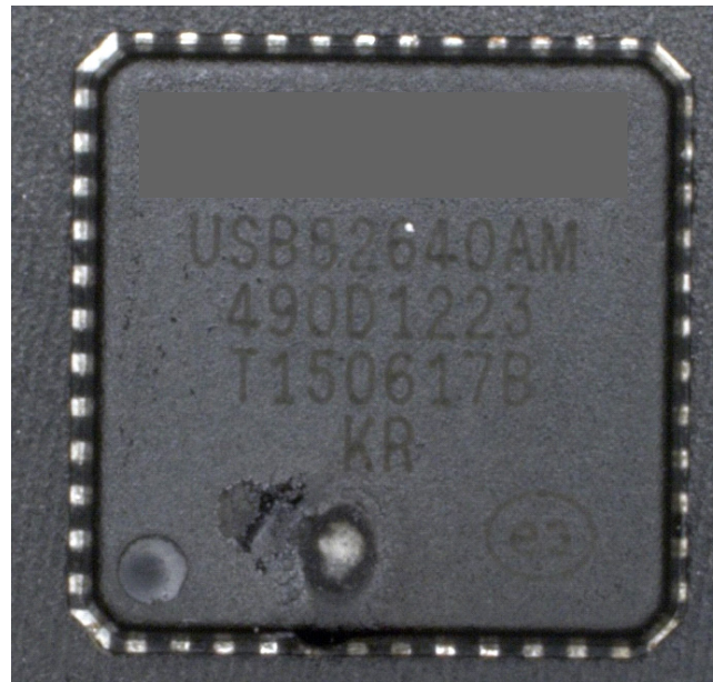
FIGURE 12: EOS DAMAGE TO PACKAGING
