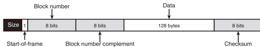
Figure 3-6. XMODEM Frame Structure
