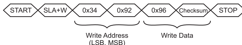
Figure 5-2. Example of a Write To Address 0x1234 With a Checksum
