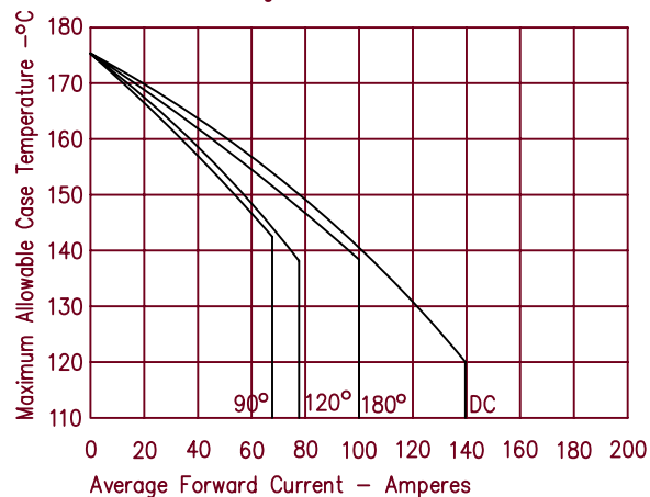
Figure 4 Forward Current Derating
