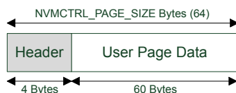
Figure 31-2. Internal Layout of an Emulated RWW EEPROM Page
