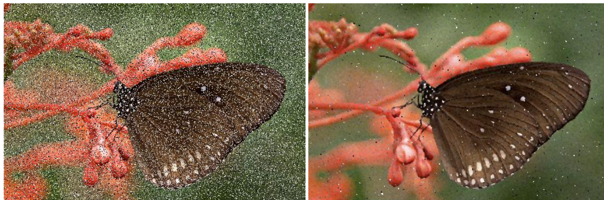
Figure 1 • Median-Based Denoising Filter Effect on a Noisy Image
