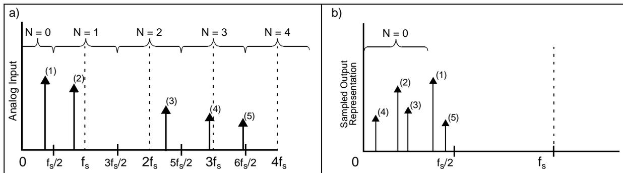
**FIGURE 6:** A system that is sampling an input signal at  $f_s$  (a) will identify signals with frequencies below  $f_s/2$  as well as above. Input signals below  $f_s/2$  will be reliably digitized while signals above  $f_s/2$  will be folded back (b) and appear as lower frequencies in the digital output.
