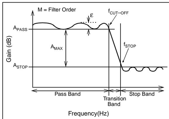
**FIGURE 2:** The key analog filter design parameters include the  $-3\text{dB}$  cut-off frequency of the filter ( $f_{\text{cut-off}}$ ), the frequency at which a minimum gain is acceptable ( $f_{\text{stop}}$ ) and the number of poles ( $M$ ) implemented with the filter.
