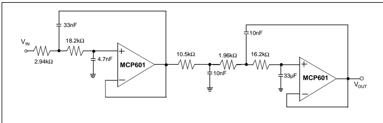
**FIGURE 14:** 5th order Bessel design implemented two Sallen-Key filters and on passive filter. This filter is designed to be an anti-aliasing filter that has a cut-off frequency of 1kHz and a stop band frequency of ~5kHz.
