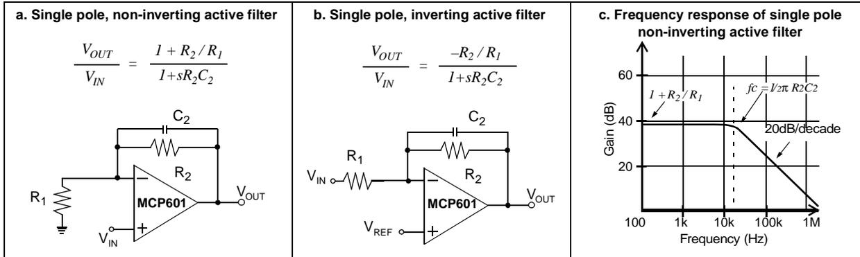
**FIGURE 9:** An operational amplifier in combination with two resistors and one capacitor can be used to implement a 1st order filter. The frequency response of these active filters is equivalent to a single pole passive low pass filter.
