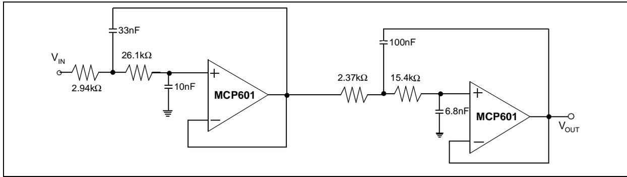
**FIGURE 17:** 4th order Butterworth design implemented two Sallen-Key filters. This filter is designed to be an anti-aliasing filter that has a cut-off frequency of 1kHz and a stop band frequency of ~5kHz.
