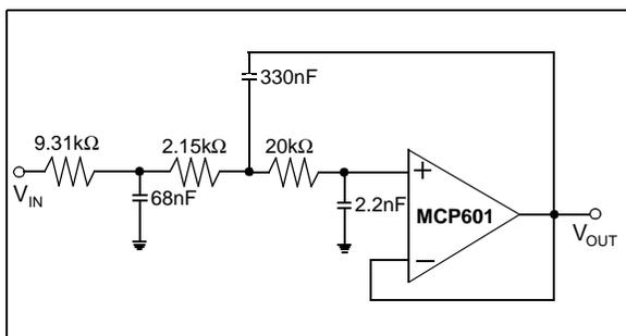
**FIGURE 15:** 3rd order Chebyshev design implemented using one Sallen-Key filter and one passive filter. This filter is designed to be an anti-aliasing filter that has a cut-off frequency of 1kHz -4db ripple and a stop band frequency of ~5kHz.
