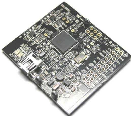
The USB Bridge is powered from the PC by using the attached USB cable. The bridge acts as a simple converter which converts the debug data packets to USB compatible data packets.
