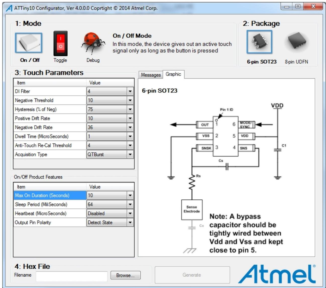
The Single Key Configurator Tool consists of several configurable parameters. They are available under QTouch Parameters and Product Features option. QTouch Parameters consist of sensor specific and global parameters related to the touch acquisition mechanism. Product Features consists of parameters which are specific to the mode of operation and have no relation to touch acquisition.
