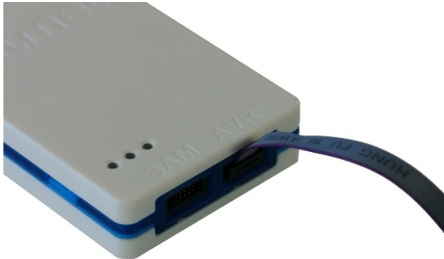
Figure 1-4. Atmel-ICE AVR Probe Connection
