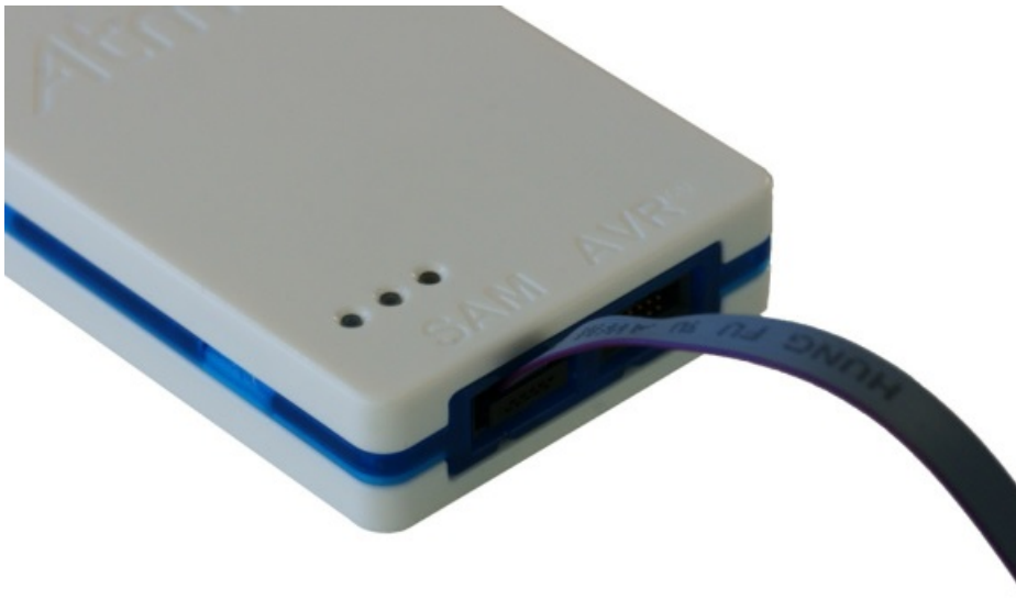
Figure 1-5. Atmel-ICE SAM Probe Connection
