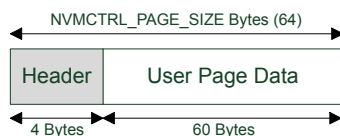
Figure 29-2. Internal Layout of An Emulated EEPROM Page
