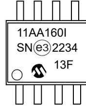
8-Lead SOIC Package Marking (Pb-Free)
