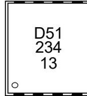
8-Lead 2x3 TDFN Package Marking (Pb-Free)
