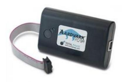
This application note explains how to use the Aardvark to generate SPI commands to the device. I2C communication is also possible, but different scripts are required. The Aardvark ribbon cable ends in a 5x2 header. Six pins – four signals and two gnds – are used for SPI communication.
