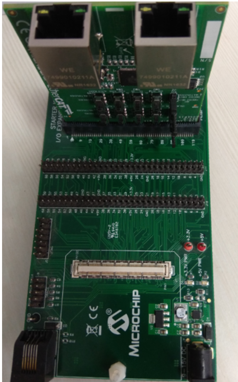
Figure 1-8. LAN9252 PICTAIL-I/O Expansion Interface
