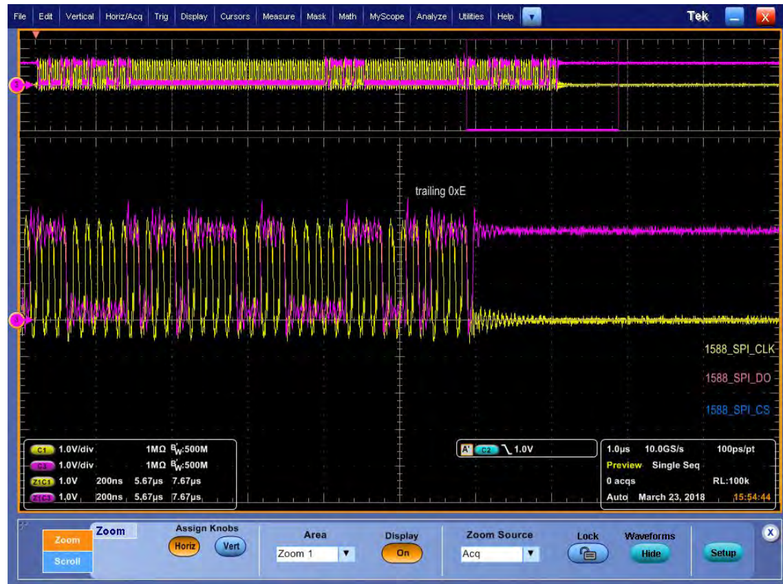
Figure 2 • SPI Timestamp Error
