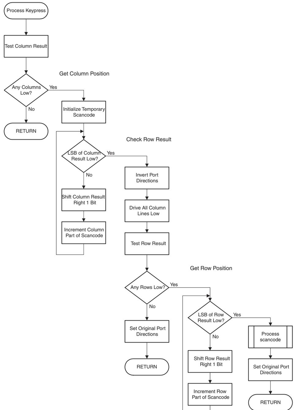
The scancode processing function first copies the generated scancode to the global variable. Then the scancode is compared to the predefined alternation key codes, updating alternation Flags accordingly. The flags are copied to the global variable. If the key wasn't an alternation key, the one-shot Flags are cleared. Finally, the update Flag is set, indicating a new keypress has been received. The procedure is shown in Figure 9.
