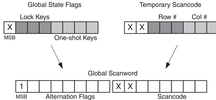
The keyboard software is implemented as an interrupt-controlled driver. The main application enters sleep mode when waiting for keypresses. The keyboard driver wakes up the AVR when a key is pressed, gets the scancode and updates the global bytes. The main application has the responsibility of reentering sleep mode, since a SLEEP instruction inside an interrupt would halt the CPU.
