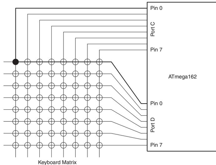
Matrix keyboards can be scanned in several ways. When only single keys are pressed, a quick method is to first select (drive low) all row lines and read the column result. Then all column lines are selected, and the row result is read. Returned column and row is combined into a unique scancode for the specific key pressed. This method is used in this application note.
