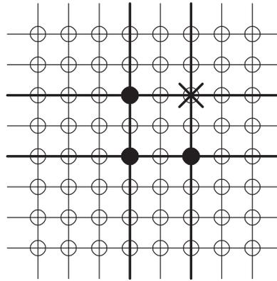
To detect a keypress and wake-up from sleep mode, the pin change interrupt on the AVR is used. Prior to entering sleep mode, all rows are selected (driven low), thus driving a column line low on any keypress in any row. (The result of a key will cause an interrupt, but will decode as “No key pressed”.)
