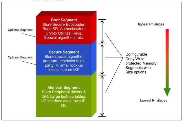
As shown in Figure 6, the Program Flash memory, RAM and EEPROM in a device featuring CodeGuard Security may be optionally segmented into three protected segments of Flash memory:
