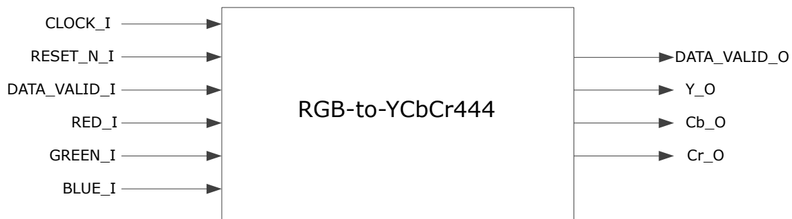
Figure 1-1. System-Level Block Diagram of RGB to YCbCr444
