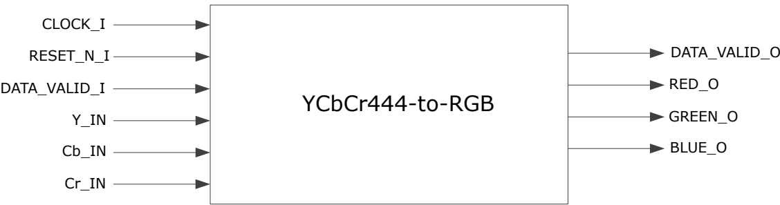
Figure 1-4. System-Level Block Diagram of YCbCr422toRGB
