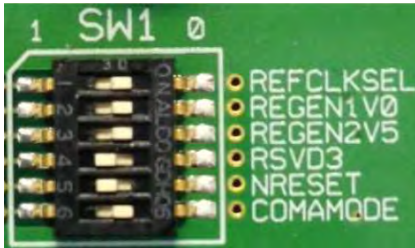
Figure 3 • SW1 Switch Control
