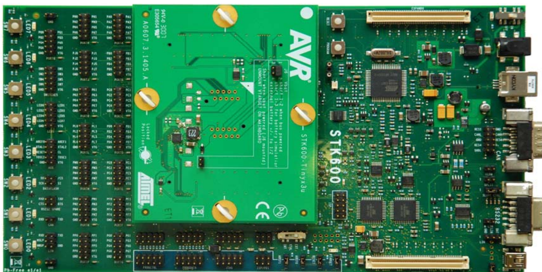
Figure 5. Demo kits such as the STK600 and ATtinyx3U top module enable developers to measure power efficiency under real-world operating conditions. These kits give developers full access to the ATtiny43U's capabilities and Atmel's comprehensive suite of proven development tools, enabling the testing of single-cell operation, power profiling of high brightness LEDs, and tuning of power thresholds to utilize the maximum capacity of cells within safe parameters.
