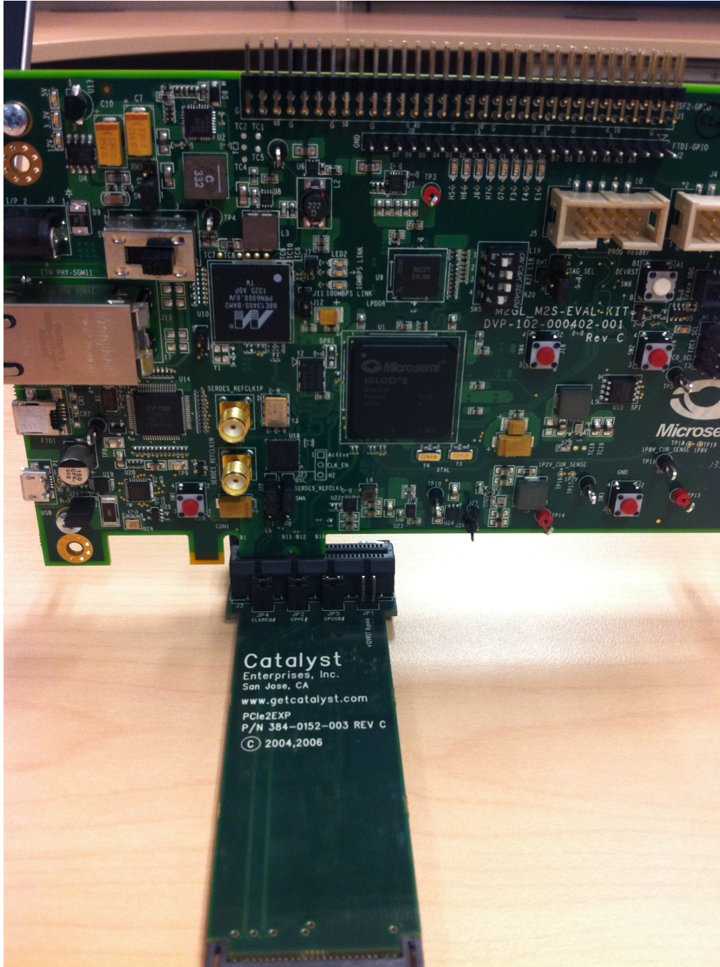
Figure 83 • Inserting the IGLOO2 Evaluation Kit PCIe Connector
