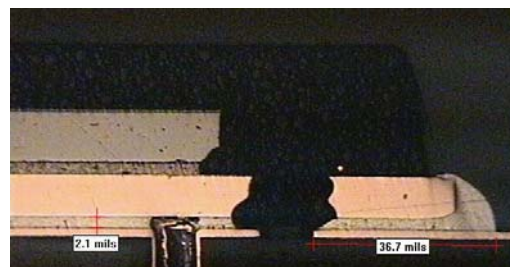
81% Paste Coverage, Encroached Via, 2.1 mil Standoff
