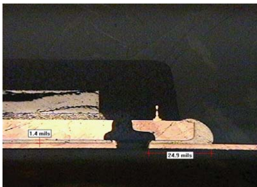
37% Paste Coverage, Plugged Via, 1.4 mil Standoff
