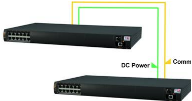
Figure 4-1. Secondary Midspan Power Backup
