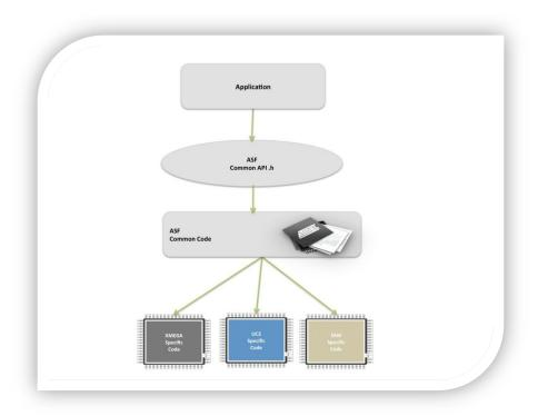
Figure 2. Example of a software framework – Atmel Software Framework architectural design
