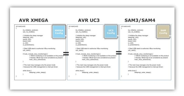
Figure 3. Identical C-code applications across Atmel's AVR, XMEGA, UC3, SAM3, SAM4 MCUs
